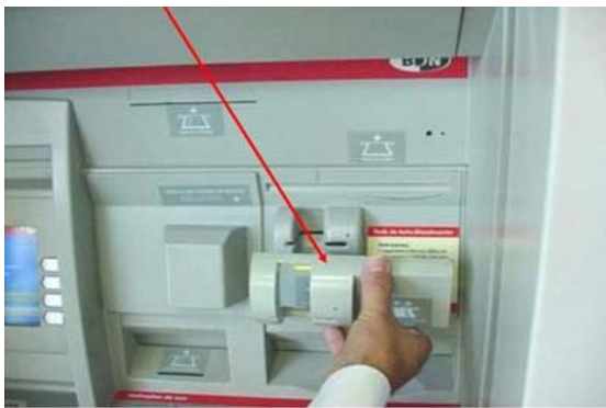
Skimming card reader placed over actual reader
