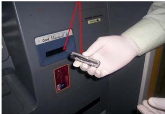
Card reader (skimmer) placed inside actual reader
