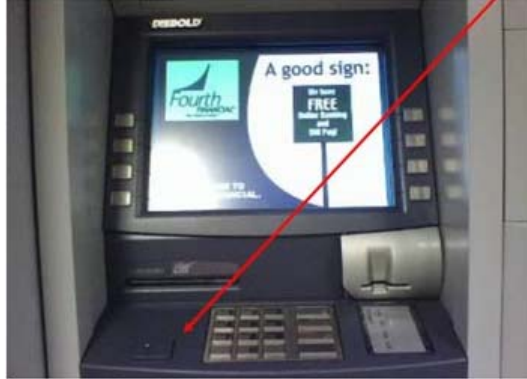
Pinhole camera concealed in plastic addition
